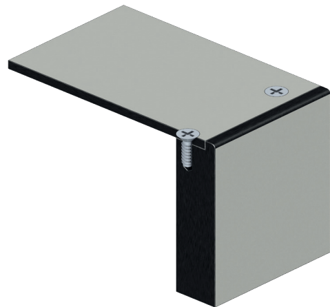
Figure 37 - Back panel finish screw-fixed with 6 mm (1/4in) Trespa® TopLab®
