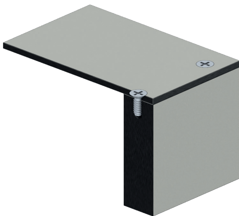
Figure 36 - Back panel finish glue-fixed with 6 mm (1/4in) Trespa® TopLab®
