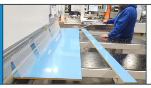
After each piece is cut, blow off any dust and/or debris to mitigate denting.
