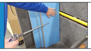
Once the piece is blown off, load into cart upright (avoid stacking HG as you run the risk of denting).
