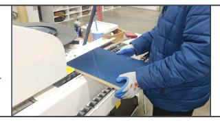
**DO NOT** press on the material when feeding to mitigate denting.
