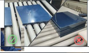
**DO NOT** stack parts on top of one another when running through Edgebander
