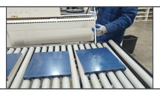
Blow off parts prior to running through Edgebander to rid of any debris that can get between belt and material.
