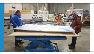
Pull foam off sheet. Load beam saw/CNC (pick up with two people to avoid sliding and denting the material).
